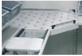
90° ball caster corner transfer. Slave board depth 700 mm, including guide rail.
