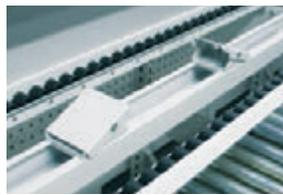
Holds the workpiece slave board securely. The tilting stopper holds the workpiece in place for the duration of the assembly. A manual release enables the transfer of the parts to the next point of assembly.
