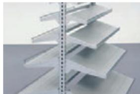
Slatted shelves for the upper work space with height adjustable in increments of 42 mm. Depths of the slatted shelves: 107, 214, 321, 428 and 535 mm. Angle from +10° to 16°.
