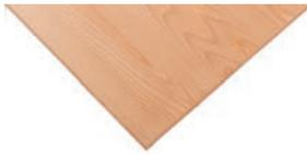
Laminated Beech plywood, glued according to BFU 100 after DIN 68705, surface treated against dirt, incl. retention holes on both sides for swivel arm elements
