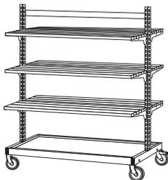
Module width 1250 mm, with 6 slatted shelves T3 (321 mm depth per side), each with stop rail, 1 base shelf
